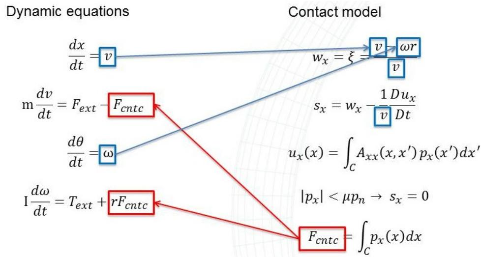
Figure 3: Illustration of the on-line coupling of MBS (dynamic equations), providing the creepage  $\xi$ , with CONTACT, providing the contact force.
