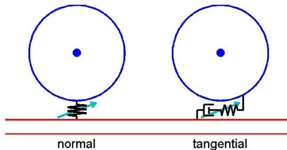
Figure 1: *Schematization of the wheel-rail rolling contact forces: acting like a spring in normal direction, Hertzian or non-Hertzian, and like a variable spring and dashpot tangentially.*
