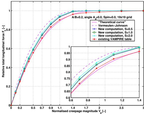
Figure 1: *Initial validation results (before model-improvement) for the new Vampire-table. Computed relative total longitudinal force  $F_x$  as a function of creepage magnitude  $V_p$ , compared to existing results.*
