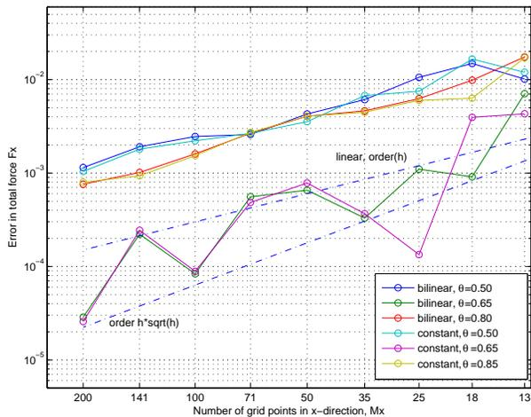
Figure 8: Convergence of  $F_x$  when refining the discretisation grid, for piecewise constant and bilinear approximations of the tractions, with varying  $\theta$ .
