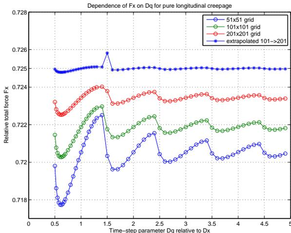
Figure 6: *Dependency of  $F_x$  on the discretisation grid and parameter  $\delta q$ , obtained using the correction of (13) at the leading edge, compare to Figure 2.*
