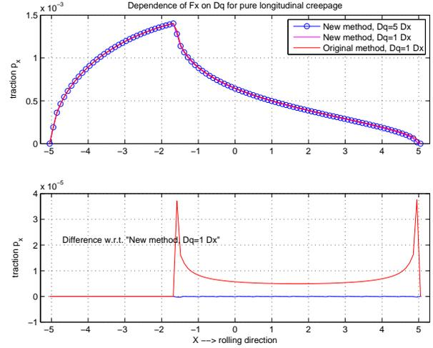
Figure 4: Results obtained using the correction of (13) at the leading edge, compare to Figure 3.
