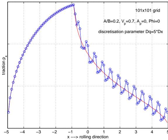
Figure 3: *An unphysical artefact in the results. Red line: correct results for time step  $\delta q = \delta x$ , blue: results for  $\delta q = 5 \cdot \delta x$ .*
