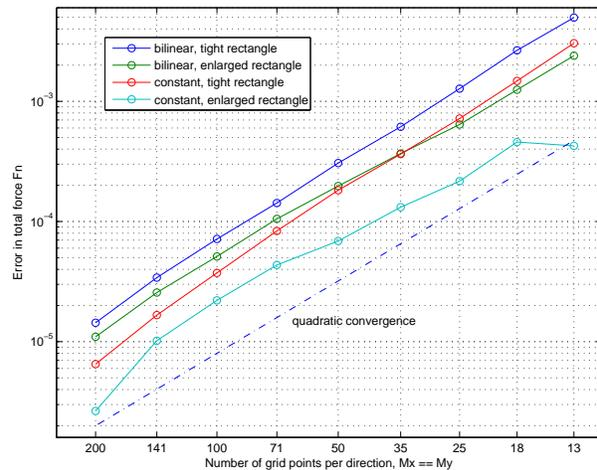
Figure 7: *Convergence of  $F_n$  when refining the discretisation grid, for piecewise constant and bilinear approximations of the tractions, and for potential contact areas that fit tightly around the true contact or that are enlarged and shifted by a half grid space.*
