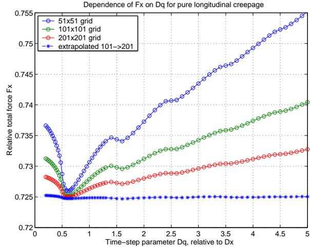
Figure 2: *Dependency of total force  $F_x$  on the discretisation grid and discretisation parameter  $\delta q$  for creepage magnitude  $V_p = 0.7$ .*
