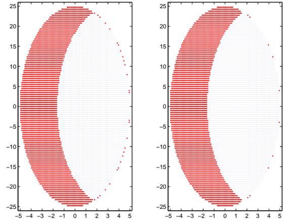
Figure 5: Adhesion and slip areas for the original (left) and new methods (right). Note that the new method has less slip at the leading edge of the contact zone.
